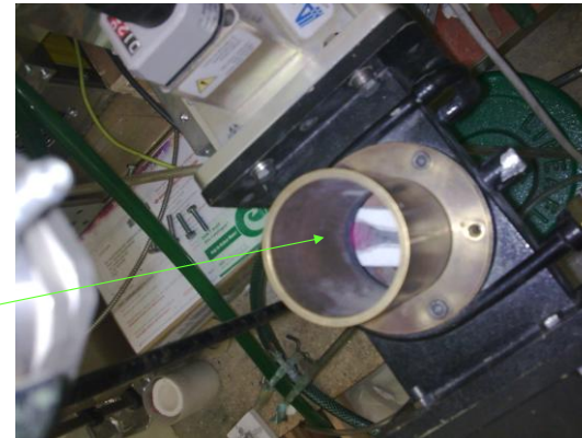
Brown part inserted in the single mode applicator based on the WR340 waveguide, showing preferential heating of the regions placed in maximum H field
