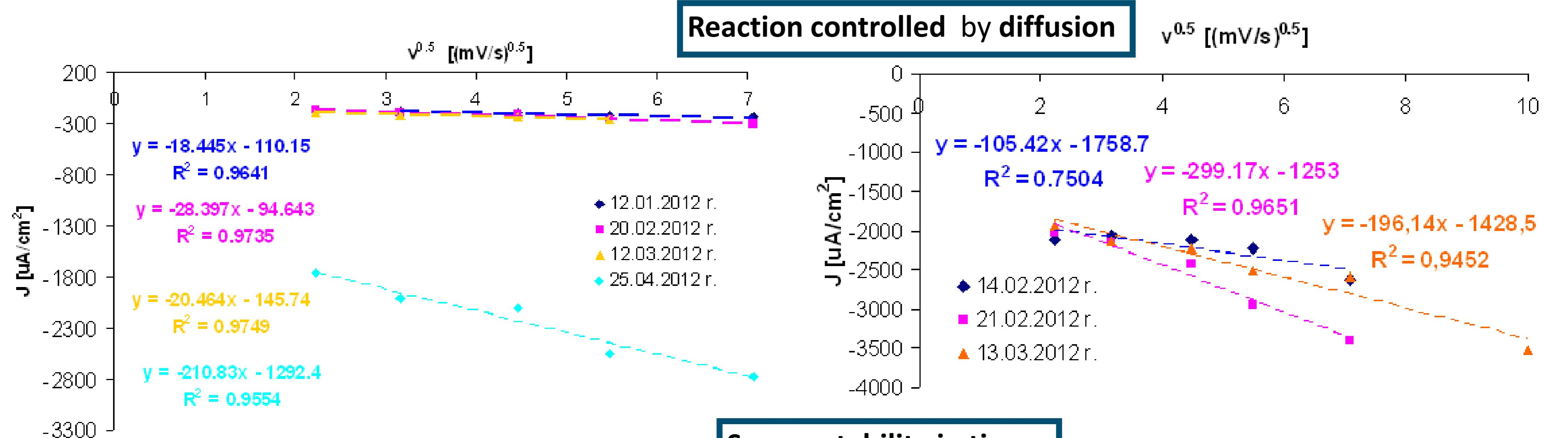
Dependences between current density and  $\text{H}_2\text{O}_2$  concentration.
