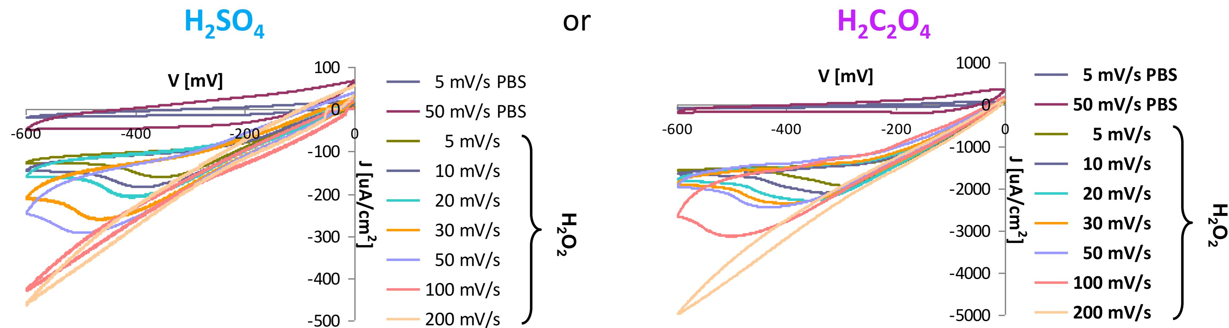
Cyclic voltamperograms of Ag nanowires electrode recorded in PBS in the absence and presence of  $\text{H}_2\text{O}_2$  at different scan rates: 5, 10, 20, 30, 50, 100, 200 mV/s.
