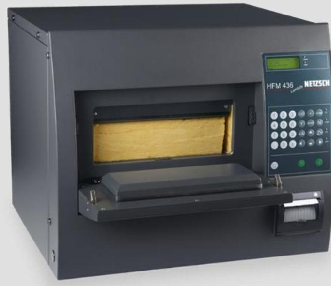
Thermal Conductivity measurements for the large samples – **insulation materials**
