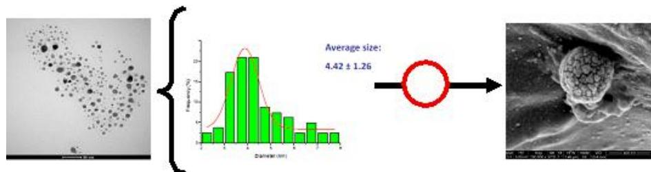
**Fig.1.** Chitosan based silver nanoparticles (<10 nm), revealing high bactericidal activity against *S. aureus*.
