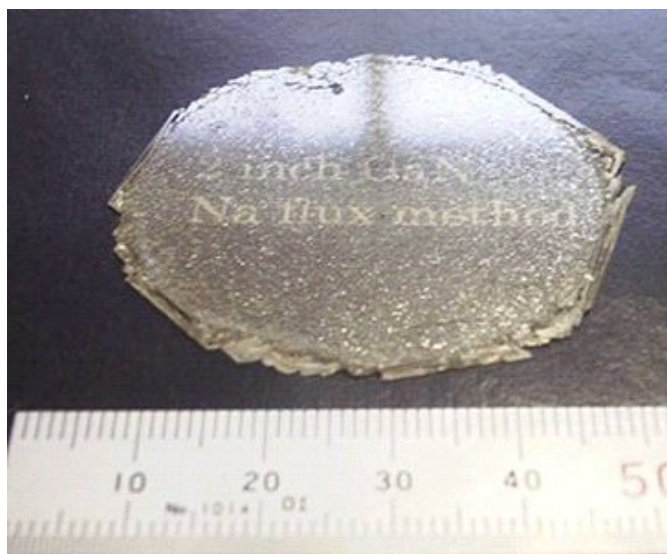
Figure 1. 2 inch GaN single crystal substrate grown by the Na flux-LPE method.
